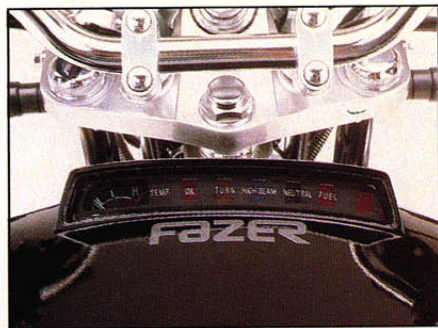
Indicator lights and coolant temperature gauge are housed in raised strip across top of airbox shelter.
